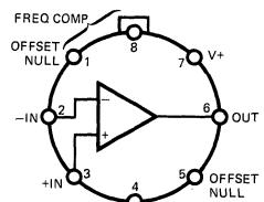
NOTE: Pin 4 connected to case.
