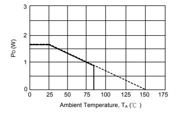
$^{*}$  On less than 3% (percentage occupied by copper foil), 70  $\times 70~mm^{2}$  , t=1.6mm glass epoxy mounting.
