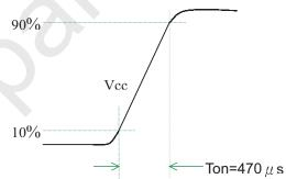
Sequence of Power-on/off and signal-on/off
