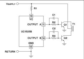
In conventional push-pull bipolar designs, forward base drive is controlled by R1-R3. Rapid turn-off times for the power devices are acheived with speed-up capacitors C, and C2.
