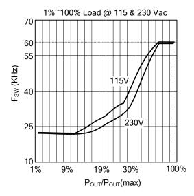
Fig.1 The relation curve between f<sub>SW</sub> and relative output power P<sub>OUT</sub> / P<sub>OUT (MAX)</sub>
