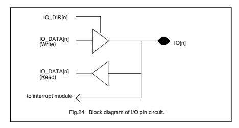
The data on the IO0-IO9 pins are feed into the interrupt control block, where they can generate an interrupt on the rising and/or falling edge of these signals.
