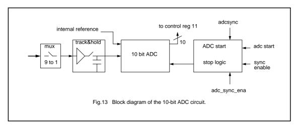
The ADC is controlled completely through the SIB interface, but the UCB1300 contains internal logic to ease the control of the ADC and to minimize the number of SIB frame read/write actions.
