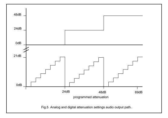
The output level can be attenuated in 3 dB steps down to -69 dB. The first 8 attenuation steps (0 to 21 dB) are implemented in the analog domain. The digital up sample filter contains a 24 dB and a 48 dB attenuation setting. This arrangement preserves the resolution, thus the 'audio quality' of the audio output signal for attenuation settings till 21 dB.
