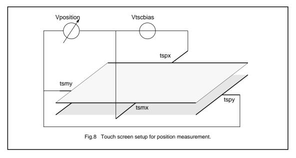
In the Y position mode the X plate and Y plate terminals are interchanged, thus the Y plate is biased while the voltage on the TSPX and/or TSMX terminal is measured.
