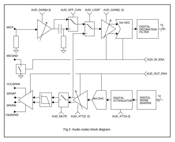
The audio sample rate ( $f_{sa}$ ) is derived from the SIB interface clock pin (SIBCLK) and is programmable through the SIB interface using AUD\_DIV[n]. The audio sample rate is given by the following equation:
