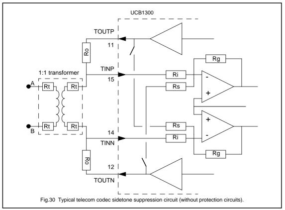
An important built-in feature of the telecom codec is the sidetone suppression circuit. The sidetone suppression circuit is activated when TEL\_SIDE\_ENA in the telecom control register B is set. The telecom input signal contains a large part of the telecom output signal, when the sidetone suppression circuit is disabled. The available dynamic range of the telecom input is occupied largely by the telecom output voltage.
