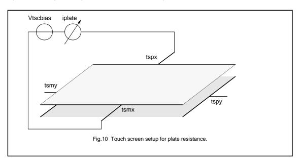
The plate resistance measurement is executed in the same way as the pressure resistance measurement. In this case only one of the two plates is biased and the other plate is kept floating. The current through the connected plate is again a direct indication of the connected resistance.
