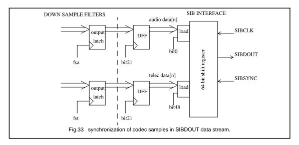
The codec samples in the SIBDOUT stream are also accompanied by a audio and telecom data valid bit (bit 30 and bit 31). These data valid flags are zero if the corresponding codec adc paths are disabled and during the start up period of the codec's, when unreliable samples are generated. By default (after reset), the data valid bits will be continuously '1' when reliable samples are generated.
