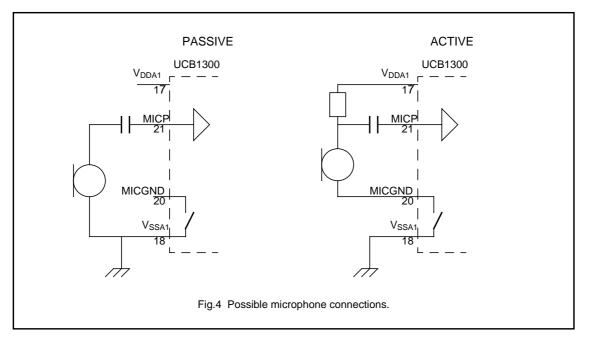
The UCB1300 audio codec input path accepts microphone signals directly, only a DC blocking capacitor is needed since the MICP input is biased around 1.4V. The 'ground' side of the microphone is either connected to the analog ground  $(V_{ssa1})$  or to the MICGND pin. The latter will decrease the current consumption of active microphones, since the MICGND pin is made Hi-Z when the audio codec input path is disabled.
