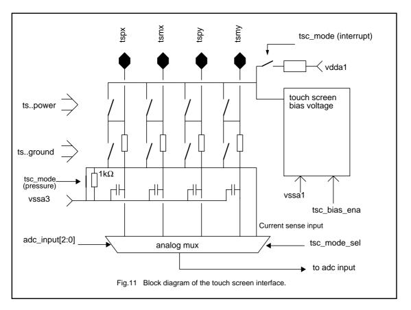
The touch screen interface connects to the touch screen by four wires: TSPX, TSMX, TSPY and TSMY. Each of these pins can be programmed to be floating, powered or grounded in the touch screen switch matrix. The setting of each touch screen pin is programmable through the touch screen control register. Possible conflicting settings (grounding and powering of a touch screen pin at the same time) are detected by the UCB1300. In that case the touch screen pin will be grounded.
