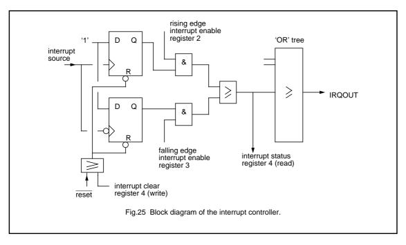
The IRQOUT pin presents the 'OR' function of all interrupt status bits and can be used to give an interrupt to the system controller.
