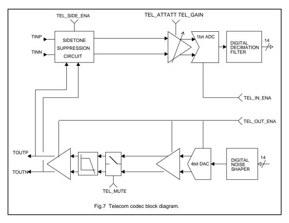
The telecom sample rate ( $f_{st}$ ) is derived from the SIB interface clock pin (SIBCLK) and is programmable through the SIB interface. The telecom sample rate is given by the following formula:
