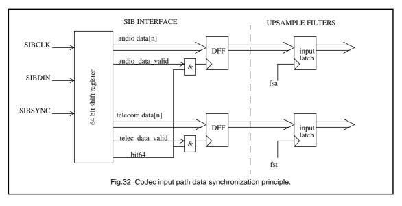
Figure 32 shows that audio and telecom data is made available for the codec up sample filters during the 64th bit in the SIB frame. This implies that the codec data has to be transferred in one of the SIB frames preceding the codec sample moment.
