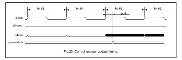
The control register data in the SIBDOUT stream is sampled just before the SIB frame is started. This implies that the returned control register data represents the 'old' control data, in case new data was provided in the SIBDIN data stream.
