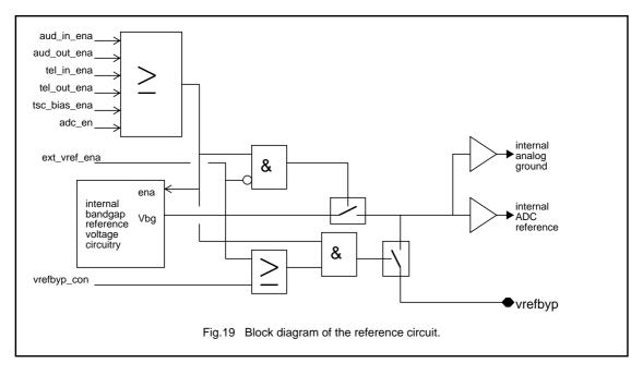
The internal reference voltage is connected to the VREFBYP pin, where an external capacitor could be connected to filter this reference voltage, if VREF\_CON (register 10) is set. THIS IS NOT RECOMMENDED since the internal impedance of the reference (several 100M $\Omega$ ) will be sensitive to board leakage and the turn on time constant will be very long.When choosing a capacitor, the internal impedance (around 50k $\Omega$ ) should be taken into account.
