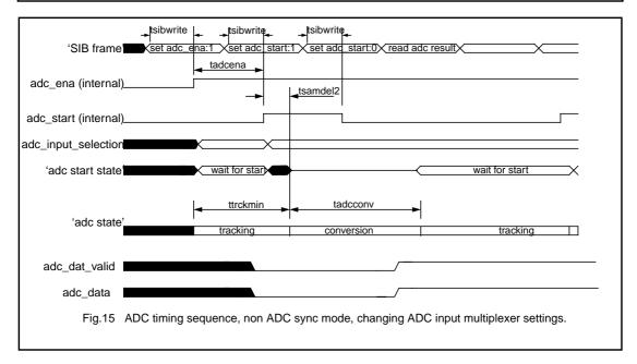
The ADC timing diagrams indicate that in the non-ADC sync mode the ADC result can be read in the SIB frame following the SIB frame with the ADC start command, if the ADC multiplexer setting is not changed. If the ADC input multiplexer setting is changed, the ADC result can be read in the second SIB frame following the SIB frame with the ADC start command.
