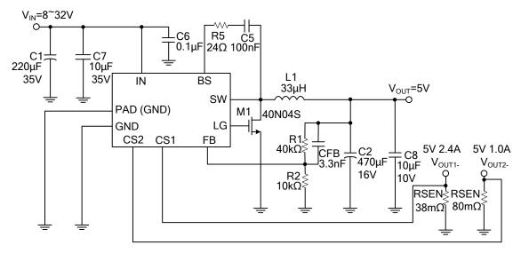
$V_{OUT} = V_{FB} \times (1 + R1/R2), \ V_{FB} = 1.00V, \ R2 \ suggest \ 1 \\ k^{\sim} 40 \\ K\Omega, \ I_{SEN} = 2.63 \\ A \ (I_{SEN} = V_{CS1} \ (0.1V)/RSEN \ (38 \\ m\Omega) \ )$
