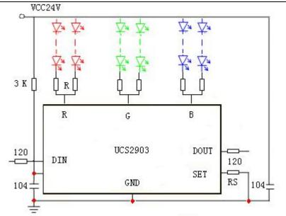
In order to prevent the damage of charged pull plug, when 24 v power supply, Din and Do all the string in a 120 ohm resistor for protection
