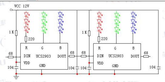
In order to prevent the damage of charged pull plug, when 12 v power supply, Din and Do all the string in a 68-80 ohm resistor for protection
