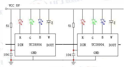
Using constant current mode can be voltage falling at the same time to achieve ideal effect of brightness and color temperature is kept constant.
