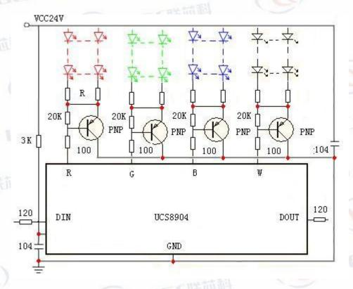
**Attention**: Shown above for the PNP transistor, 9012,8550 is work In order to prevent the damage of charged pull plug, when 24 v power supply, Din and Do all the string in a 120 ohm resistor for protection
