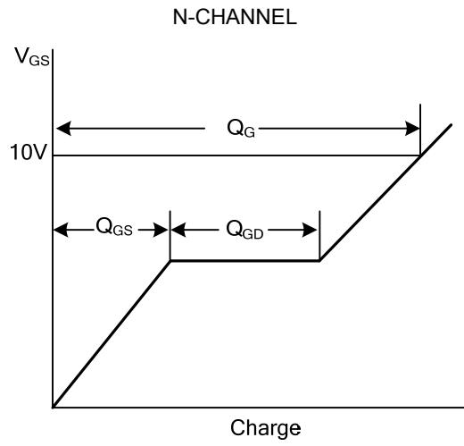
Gate Charge Waveforms
