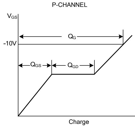
Gate Charge Waveforms
