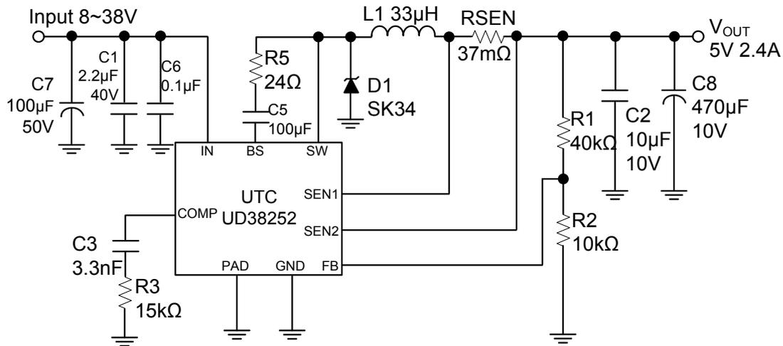
$$V_{OUT} = V_{FB} \times (1 + R1/R2), \quad V_{FB} = 1.00V, \quad R2 \text{ suggest } 1K \sim 30K\Omega$$
