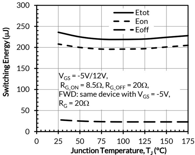
Figure 21. Clamped inductive switching energy vs. junction temperature at  $V_{DS} = 800V$  and  $I_D = 13A$
