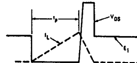
Fig. 16 - Clamped Inductive Waveforms
