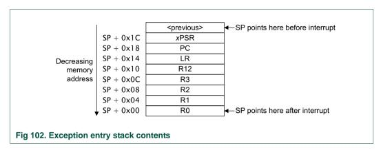
Immediately after stacking, the stack pointer indicates the lowest address in the stack frame. The stack frame is aligned to a double-word address.
