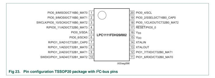
Table 166. LPC1110/11/12 pin description table (SO20 and TSSOP20 package with I<sup>2</sup>C-bus pins)
