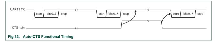
While starting transmission of the initial character, the  $\overline{\text{CTS}}$  signal is asserted. Transmission will stall as soon as the pending transmission has completed. The UART will continue transmitting a 1 bit as long as  $\overline{\text{CTS}}$  is de-asserted (high). As soon as  $\overline{\text{CTS}}$  gets de-asserted, transmission resumes and a start bit is sent followed by the data bits of the next character.
