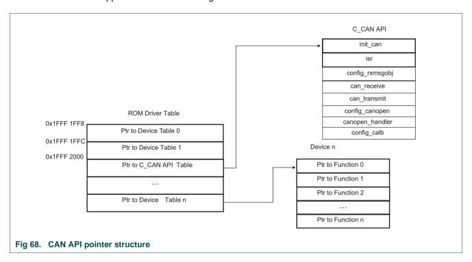
In C, the structure with the function list that is referenced to call the API functions looks as follows:
