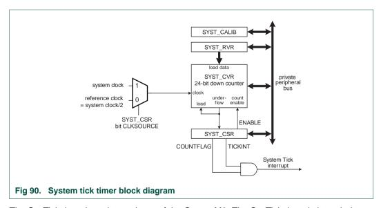
The SysTick timer is an integral part of the Cortex-M0. The SysTick timer is intended to generate a fixed 10 millisecond interrupt for use by an operating system or other system management software.
