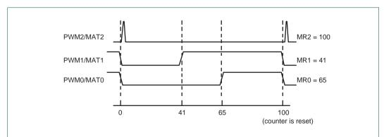
Fig 69. Sample PWM waveforms with a PWM cycle length of 100 (selected by MR2) and MAT2:0 enabled as PWM outputs by the PWCM register.
