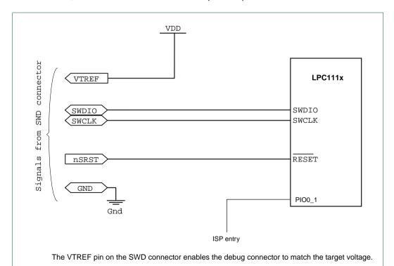
Fig 94. Connecting the SWD pins to a standard SWD connector
