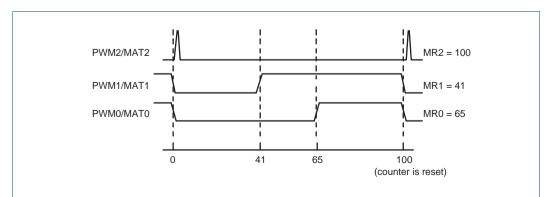
Fig 73. Sample PWM waveforms with a PWM cycle length of 100 (selected by MR2) and MAT2:0 enabled as PWM outputs by the PWCM register.
