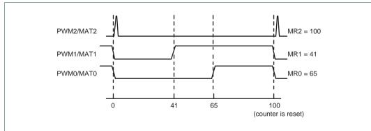
Fig 83. Sample PWM waveforms with a PWM cycle length of 100 (selected by MR2) and MAT2:0 enabled as PWM outputs by the PWMC register.
