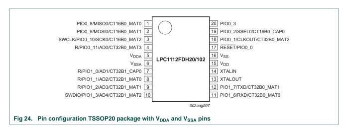
Table 167. LPC1112 pin description table (TSSOP20 with V<sub>DDA</sub> and V<sub>SSA</sub> pins)
