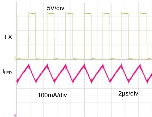
Steady State Waveforms ( V_{IN}=16V , 3 LEDs, L1=100\mu H , R_s=0.33\Omega )
