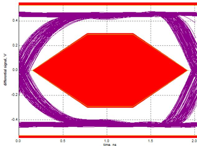
**Figure 4 USB Eye Diagram**
