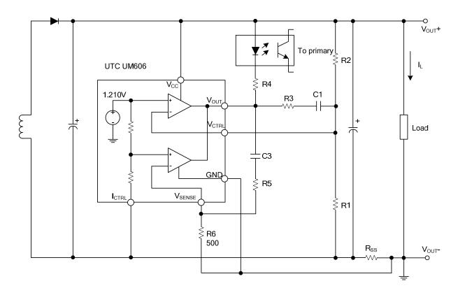
$$\begin{split} V_{OUT} = & \left[ V_{REF} + \left( I_L \times R_{SS} \right) \right] \times \frac{R1 + R2}{R1} - \left( I_L \times R_{SS} \right) \ \ \, \text{(V)} \end{split}$$
