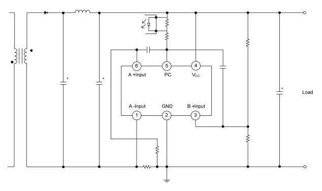
In the above application schematic, the UTC **UM607** is used on the secondary side of a flyback adapter (or battery charger) to provide an accurate control of voltage and current. The above feedback loop is made with an optocoupler.
