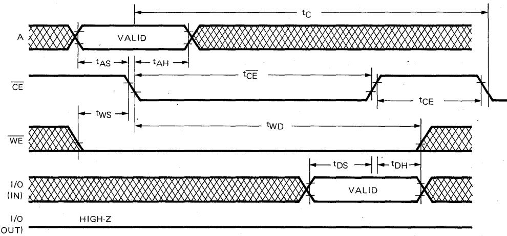
**READ MODIFY WRITE CYCLE TIMING DIAGRAM**
