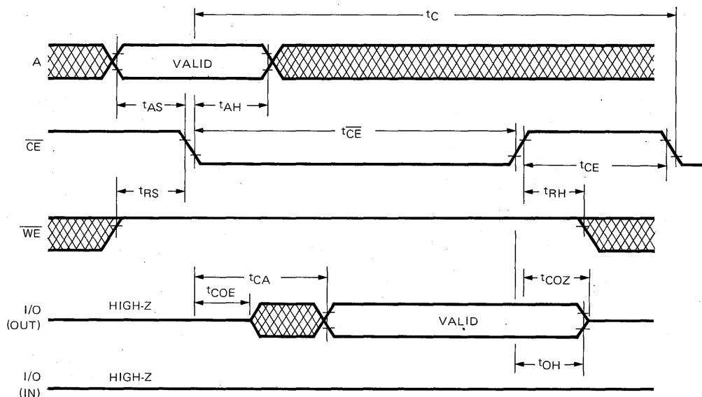
**WRITE CYCLE TIMING DIAGRAM**
