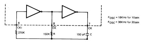
This oscillator consists of two inverters, the oscillator frequency is controlled by external RC components  $R_{CKI} = 270 \text{ K}$   $R_{CK} = 150 \text{ K}$   $C_{CKO} = 150 \text{ pF}$
