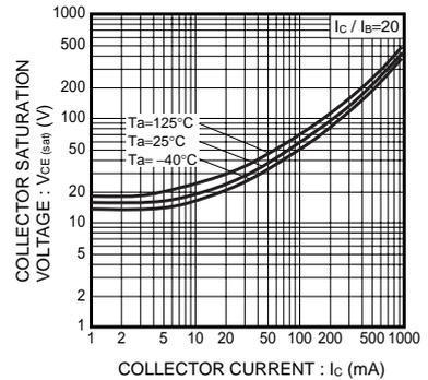
Fig.3 Collector-Emitter Saturation Voltage vs. Collector Current (I)
