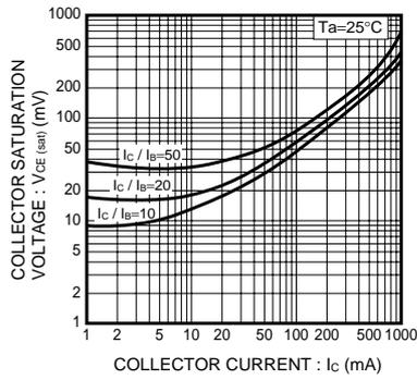
Fig.4 Collector-Emitter Saturation Voltage vs. Collector Current (II)
