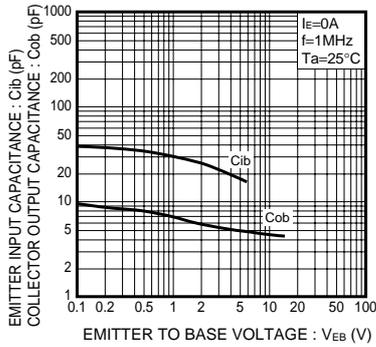
Fig.7 Collector Output Capacitance vs. Collector-Base Voltage
