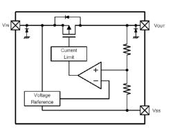
\*Diodes inside the circuit are an ESD protection diode and a parasitic diode.
