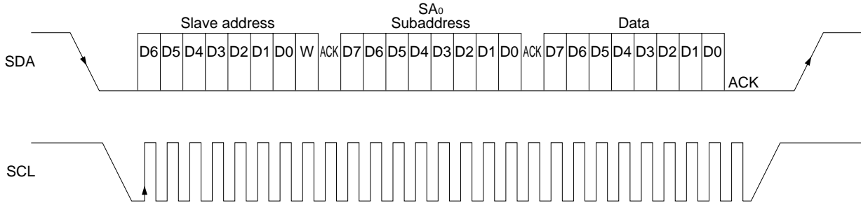
Figure 3-4. Example of Data Transfer in Write Mode
