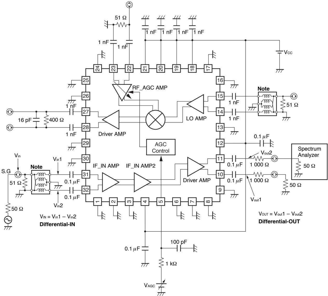
**Note** Balun Transformer : TOKO 617DB-1674 B4F (Double balanced type)
