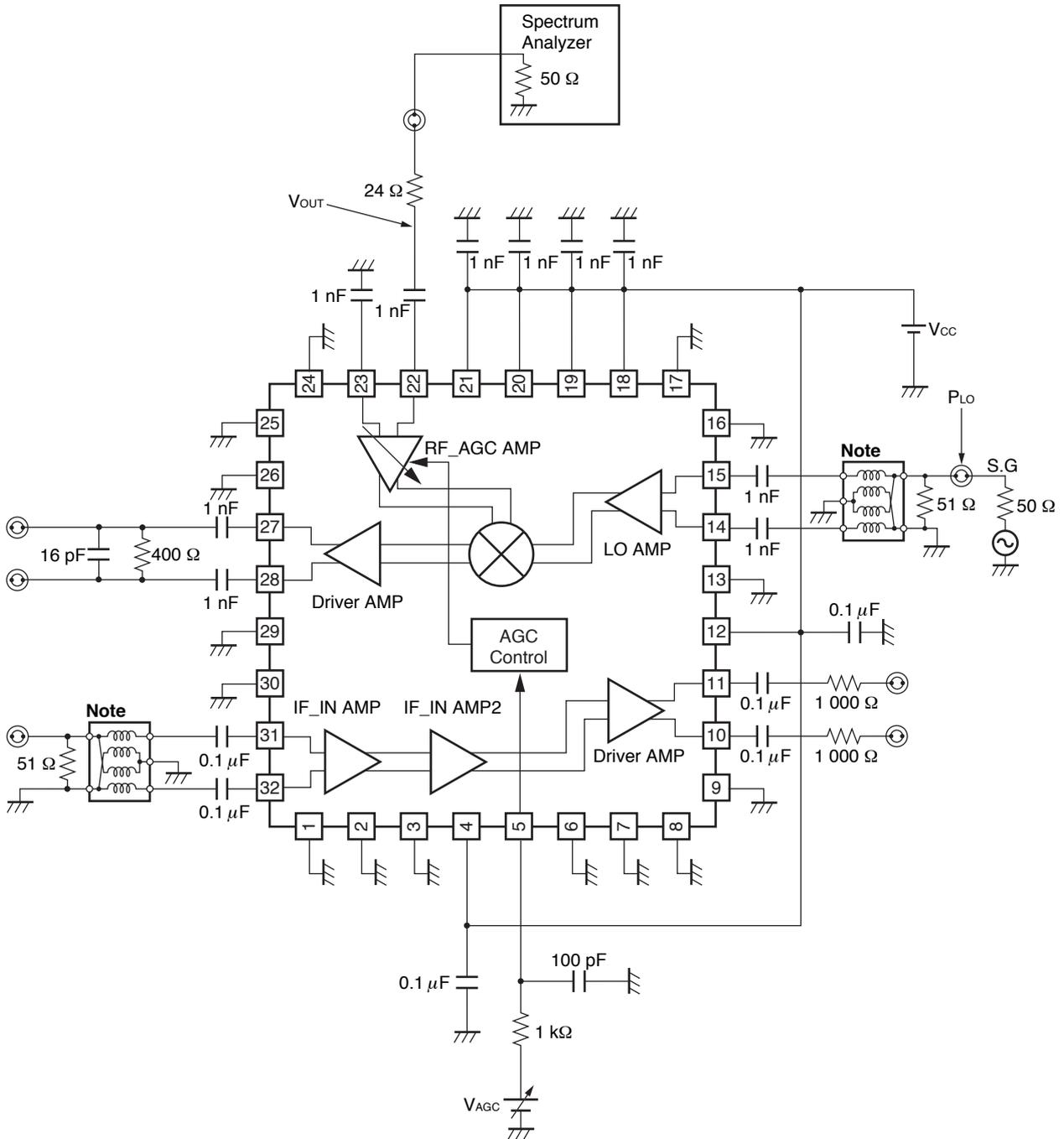
**Note** Balun Transformer : TOKO 617DB-1674 B4F (Double balanced type)
