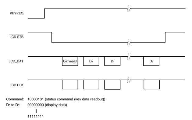
After the status command is send, key data is read from the LCD\_DAT pin.
