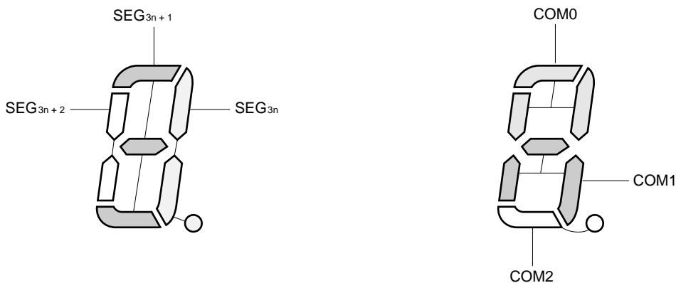
Figure 13-7: 3-Time-Division LCD Display Pattern and Electrode Connections
