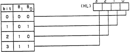
S Example: Whether bit 3 of data memory (10H) is 0 is tested. LHLI 10H :HL=10H SKMBF 3 :SKIP IF (10H)<sub>3</sub>=0 JMP ERR :JUMP TO ERR OK: SKAEM (Skip if A Equals Memory)
