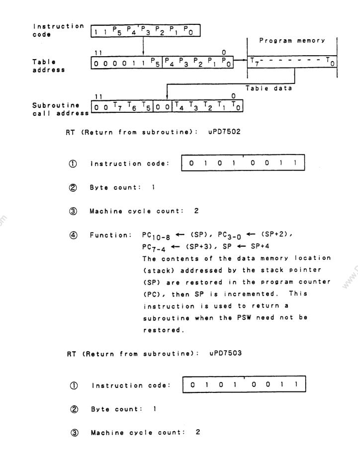
(4) Function:  $PC_{11-8} \leftarrow (SP)$ ,  $PC_{3-0} \leftarrow (SP+2)$ ,  $PC_{7-4} \leftarrow (SP+3)$ ,  $SP \leftarrow SP+4$ The contents of the data memory location (stack) addressed by the stack pointer (SP) are restored in the program counter (PC), then SP is incremented.
