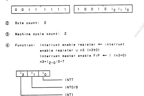
The contents of the interrupt enable register are ORed with 3-bit immediate data n3, and the result is stored in the interrupt enable register. This means that by setting the bit specified for a desired interrupt to 1, the associated one or more interrupts are enabled.
