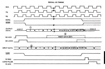
1 Data clocked out on falling edge of SCK.
