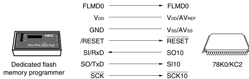
Figure 25-10. Communication with Dedicated Flash Memory Programmer (CSI10)
