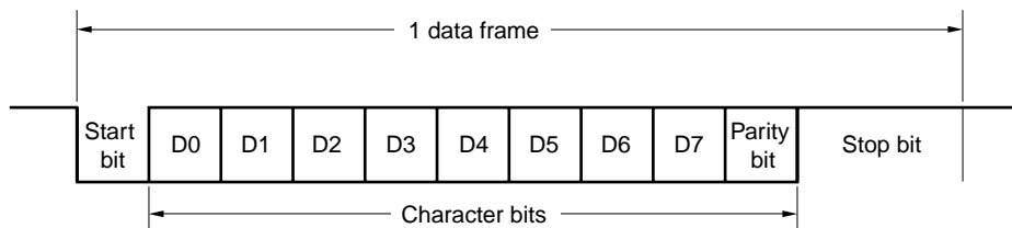
Figure 14-6. Format of Normal UART Transmit/Receive Data
