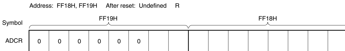
Figure 9-6. Format of 10-Bit A/D Conversion Result Register (ADCR)
