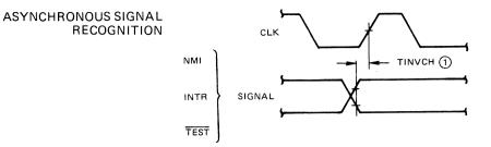
NOTE: (1) Setup requirements for asynchronous signals only to guarantee recognition at next CLK.
