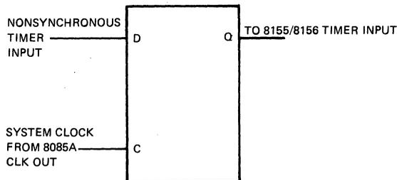
When using the timer of the 8155/8156 care must be taken if the timer input is an external, nonsynchronous event. To sync this signal to the system clock the flip-flop shown should be used.
