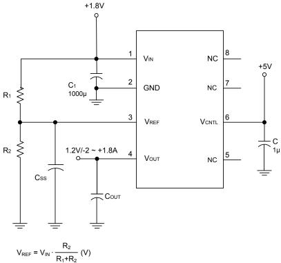
$$V_{REF} = V_{IN} \cdot \frac{R_2}{R_1 + R_2} (V_{OUT})$$
