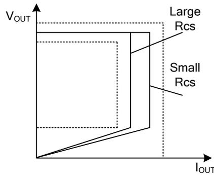
Figure 3. Adjustable output power by changing  $R_{cs}$
