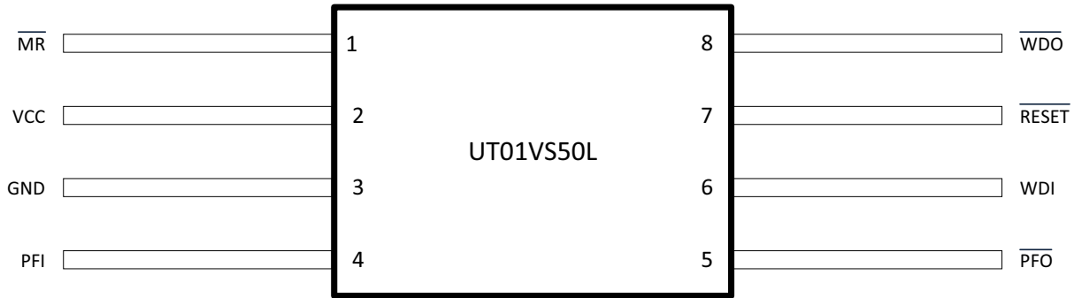
Figure 2. UT01VS50L Pin Configuration
