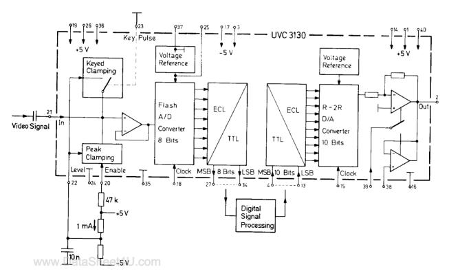
Fig. 12: Operation with peak clamping
