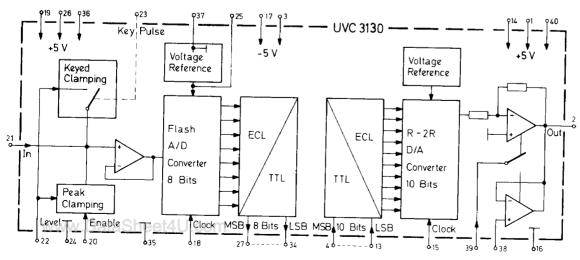
Fig. 1: UVC 3130 block diagram
