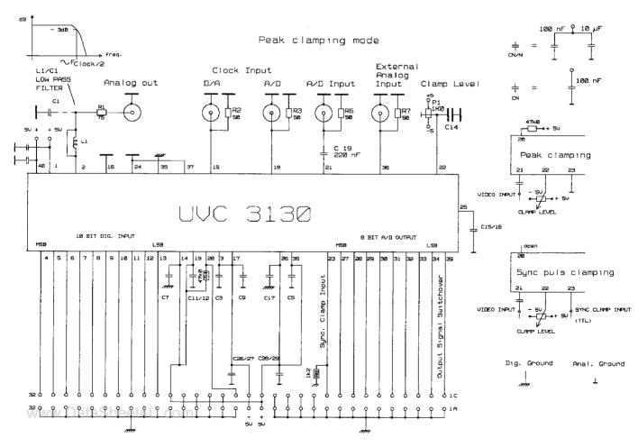
Fig. 14: Application diagram including power supply and associated decoupling elements.
