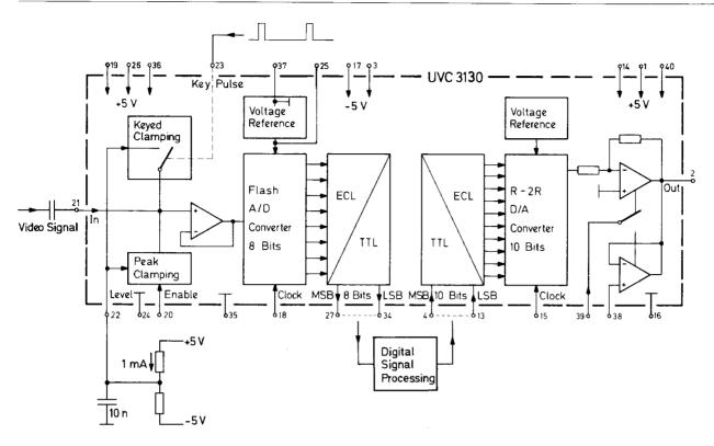
**Fig. 13:** Operation with keyed clamping During the key pulse, the input signal must have that level to which it is to be clamped. Pin 20 must not be connected.
