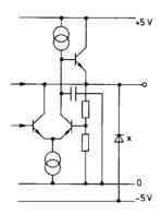
Fig. 9: Pin 25, Reference Voltage Pin
