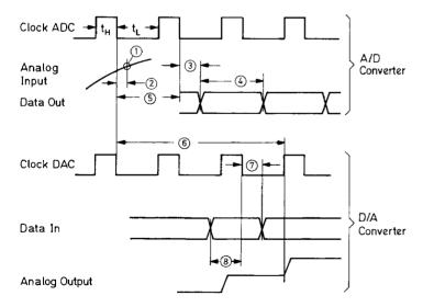
Fig 3: Timing diagram of the UVC 3130 A/D-D/A Converter
