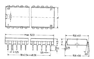
Fig. 2: UVC 3130 in 40-pin Dil Plastic Package, 20 B 40 according to DIN 41870
