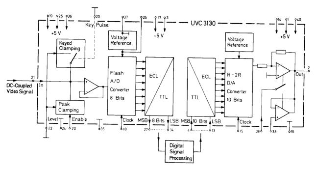
Fig. 11: Operation without clamping of the input signal Pin 20 must not be connected.
