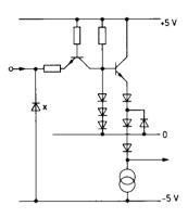
Fig. 5: Pins 4 to 13 and 15, Inputs
