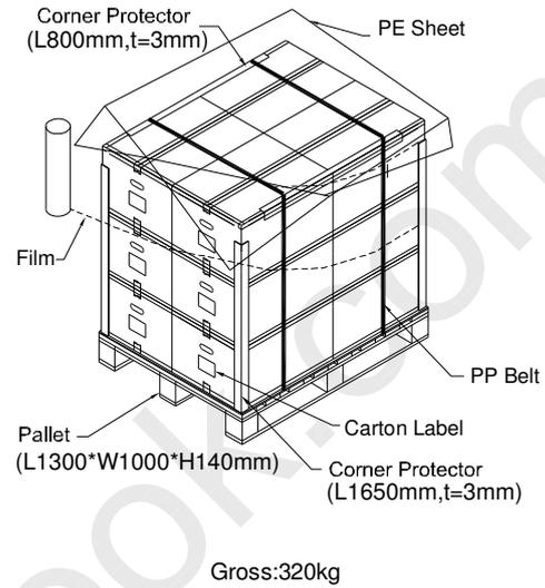
Figure.9-2 Packing Method
