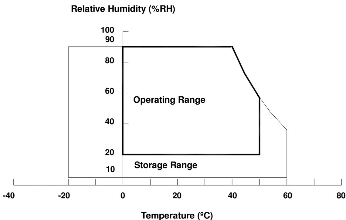
Note (2) The maximum operating temperature is based on the test condition that the surface temperature of display area is less than or equal to 65 °C with LCD module alone in a temperature controlled chamber. Thermal management should be considered in your product design to prevent the surface temperature of display area from being over 65 °C. The range of operating temperature may degrade in case of improper thermal management in your product design.
