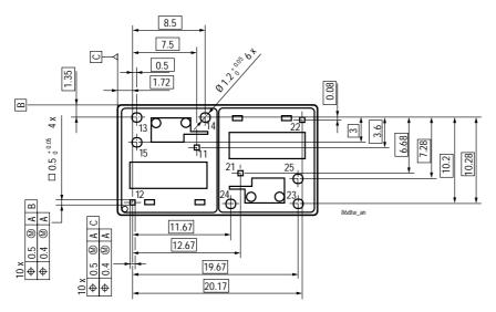
Remark: Positional tolerances according to DIN EN ISO 5458
