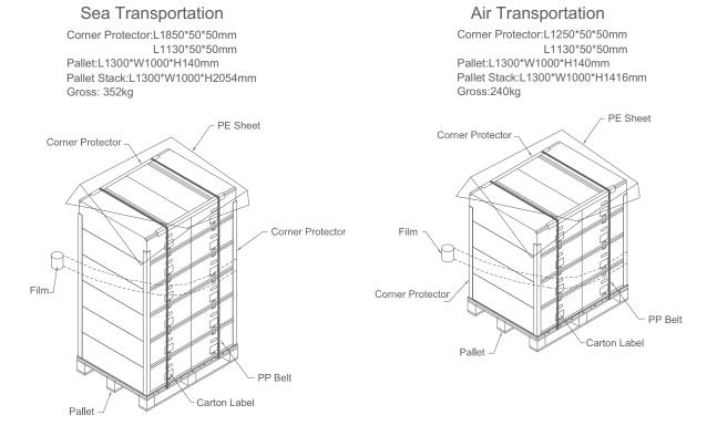
Figure.9-2 packing method
