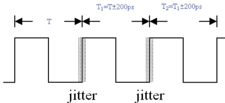
Note (4) The SSCG (Spread spectrum clock generator) is defined as below figures.
