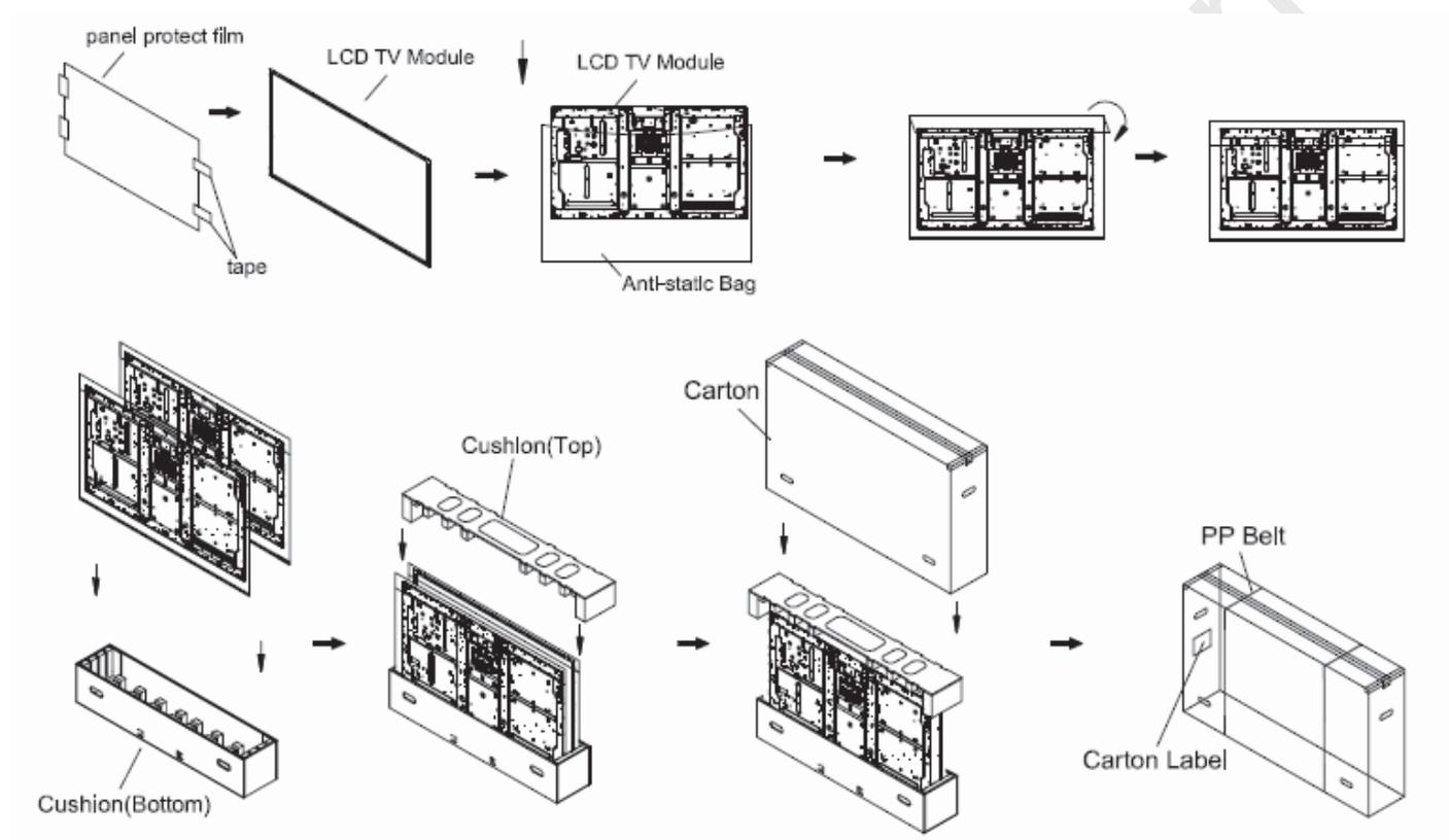
Figure 10-1 packing method
