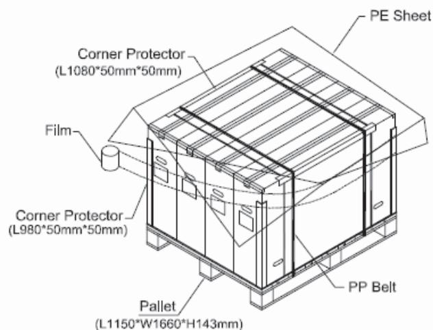
Figure 10-2 packing method
