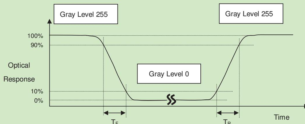
The driving signal means the signal of gray level 32, 64, 96, 128, 160, 192 and 224
