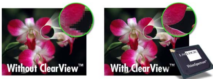
Example of improved picture using ClearView™ Deinterlacing.
