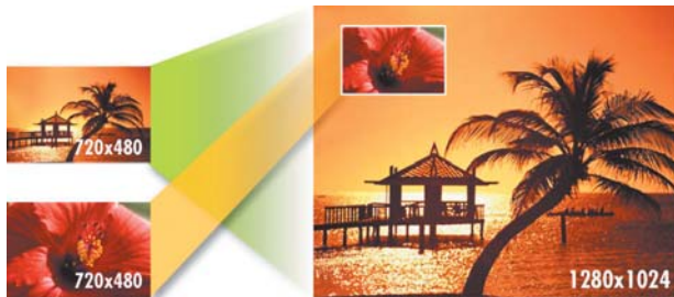
Example of main and PIP scaling for SXGA display.
