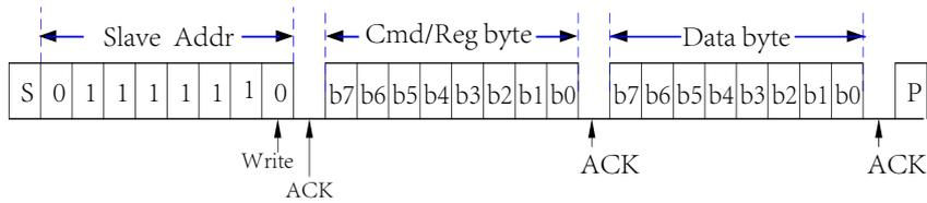
Note: If the byte after the Slave address is a command code, the byte after the command code is ignored.
