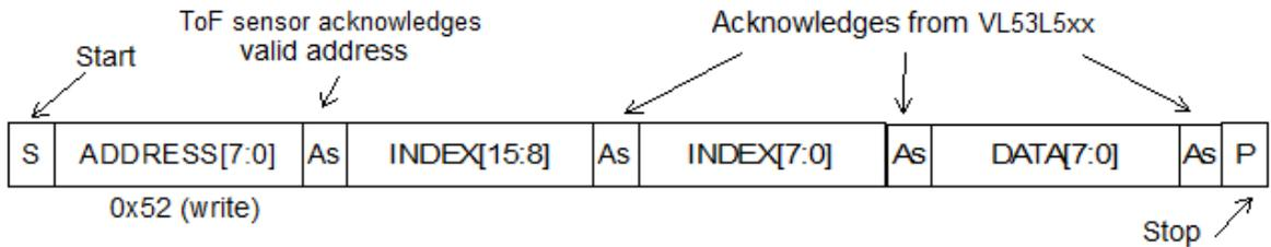
As data are received by the target, they are written bit by bit to a serial/parallel register. After each data byte has been received by the target, an acknowledge is generated, the data are then stored in the internal register addressed by the current index.
