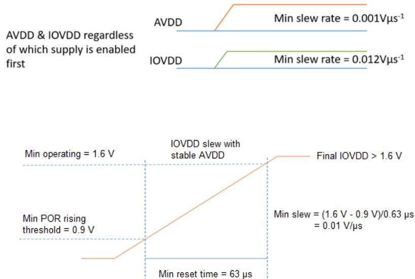
*Note:* The minimum reset time is the minimum time required for the device ROM to load and boot up after IOVDD reaches the POR rising threshold. The supply must have reached the minimum operating level (1.6 V) within this time.
