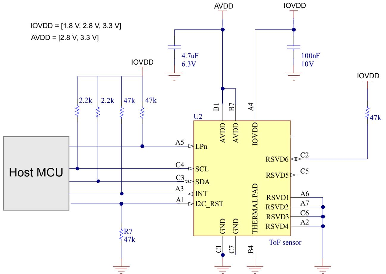
Note: Capacitors on the external supplies (AVDD and IOVDD) should be placed as close as possible to the module pins.
