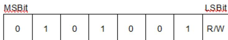
All serial interface communications with the ToF sensor must begin with a start condition. The VL53L7CH module acknowledges the receipt of a valid address by driving the SDA wire low. The state of the read/write bit (lsb of the address byte) is stored and the next byte of data, sampled from SDA, can be interpreted. During a write sequence, the second byte received provides a 16-bit index, which points to one of the internal 8-bit registers.
