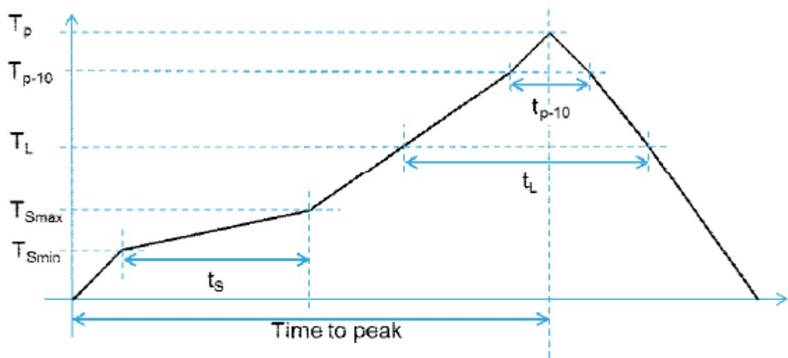
*Note:* The component should be limited to a maximum of three passes through this solder profile.
