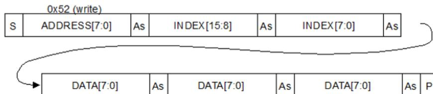
**Figure 15. VL53L7CH data format (sequential read)**
