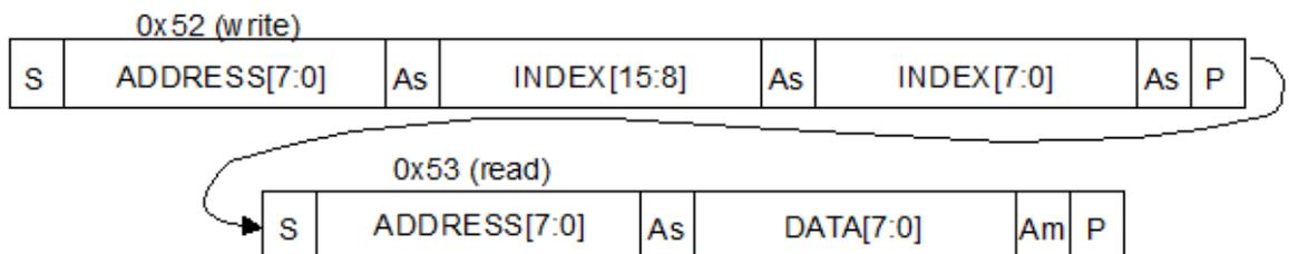
At the end of each byte, in both read and write message sequences, an acknowledge is issued by the receiving device (that is, the VL53L7CH for a write and the host for a read).
