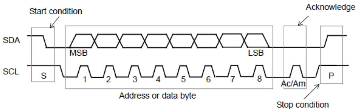
Information is packed in 8-bit packets (bytes) always followed by an acknowledge bit, Ac for VL53L7CH acknowledge and Am for controller acknowledge (host bus controller). The internal data are produced by sampling SDA at a rising edge of SCL. The external data must be stable during the high period of SCL. The exceptions to this are start (S) or stop (P) conditions when SDA falls or rises respectively, while SCL is high.
