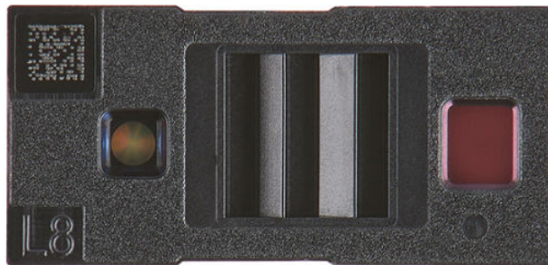
Figure 34. 2D marking product code on module cap
