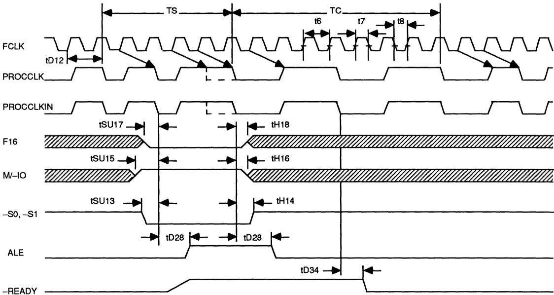
**Note:** Timing is shown for an off-board memory cycle. The same clock transitions will occur if M-I/O is sampled low, regardless the state of F16.
