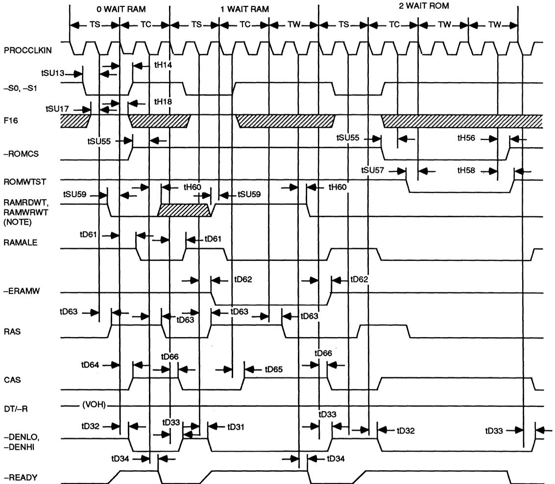
**Note:** Although RAMRDWT and RAMWRWT can be changed dynamically for each memory cycle, care must be taken to never allow RAMRDWT to be high and RAMWRWT to be low at the same time for more than 60 ns. This results in zero wait state write cycles and one wait state read cycles. This was determined to be an unrealistic operating mode and is used to put the VL82C201 into a test mode that will disrupt normal system operation.
