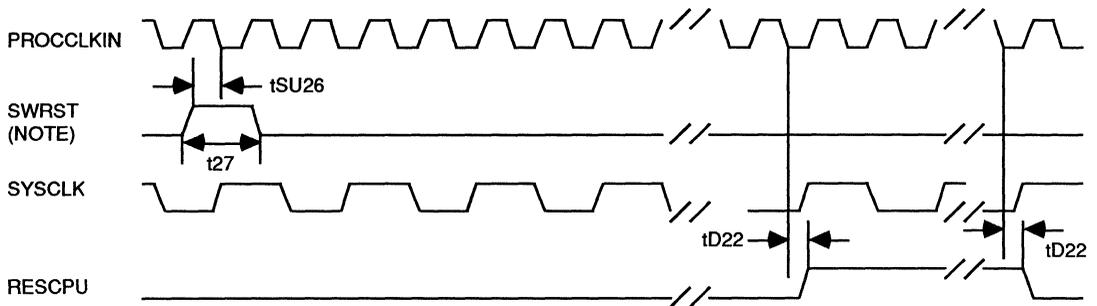
**Note:** POWERGOOD and SWRST are asynchronous inputs. This specification is given for testing purposes only, to assure recognition at a specific PROCCLKIN edge.
