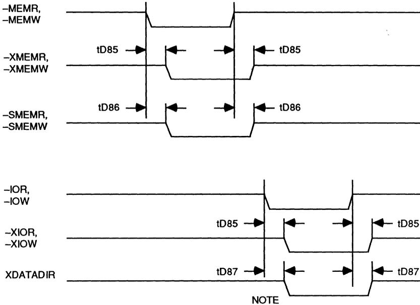
**Note:** XDATADIR goes low only for  $\overline{\text{IOR}}$  when  $\text{XA9}$ ,  $\text{XA8}$  are low and  $\overline{\text{NPCS}}$  is not active.
