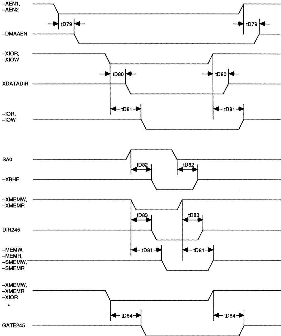
**BUS MASTER MODE TIMING WAVEFORM**
