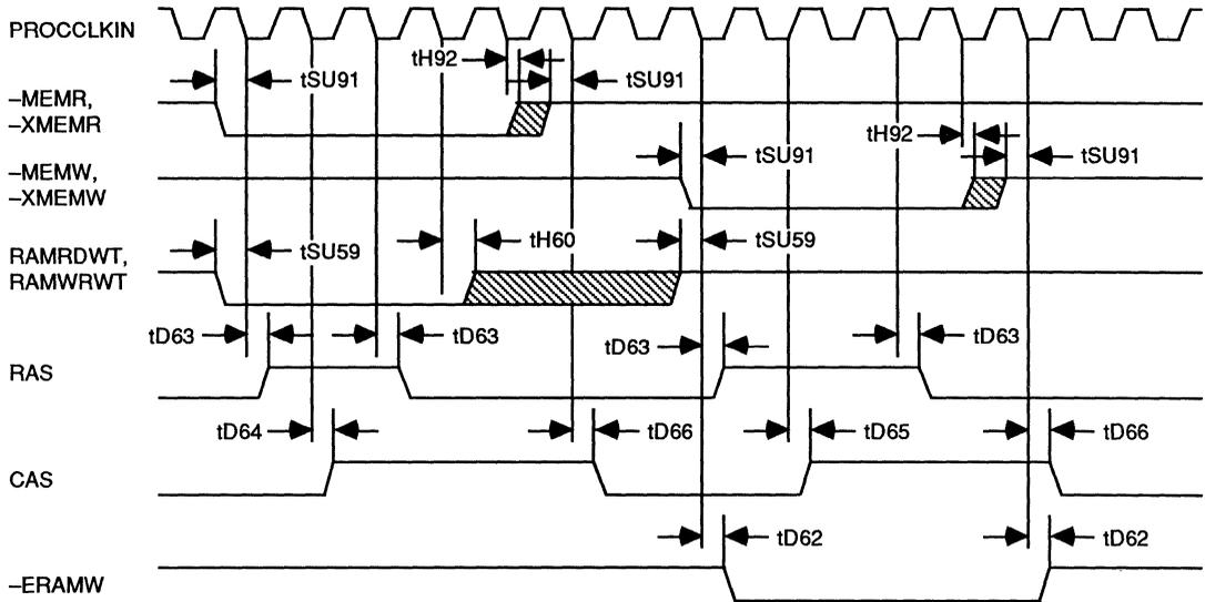
BUS CONTROL TIMING WAVEFORMS DURING DMA OR MASTER MODES
