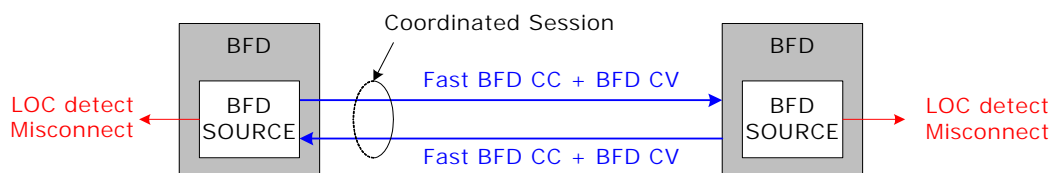
Figure 86 • BFD Coordinated Mode
