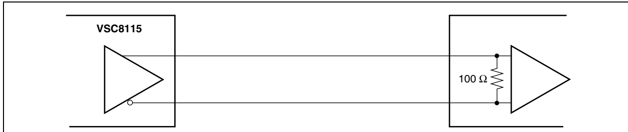
Figure 4. High-Speed Outputs, LVDS Termination
