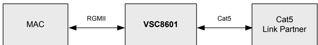
Figure 3. RGMII to Cat5 Block Diagram
