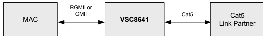
Figure 3. RGMI or GMI to Cat5 Block Diagram
